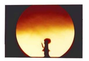
...this obstruction blocks those light rays that would have fallen on the top portions of the screen but does not affect the brightness of the screen below. The obstruction basically casts a shadow of itself on the screen. Some of the light is actually eliminated from reaching the top of the screen.
