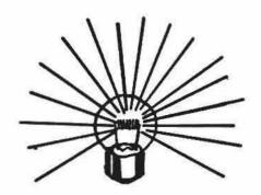
For all test methods, a light source is required. Light will emanate from this source in all directions. For now we will deal only with a "point" source, although a true point source is often not obtainable or desirable.
