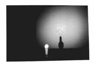
A big advantage of the shadowgraph system is that it is relatively cheap to set up and that it can deal with subjects of relatively large size. Attempts to increase the system sensitivity invariably raise the cost and the improved versions usually start to become very similar to Schlieren systems.
